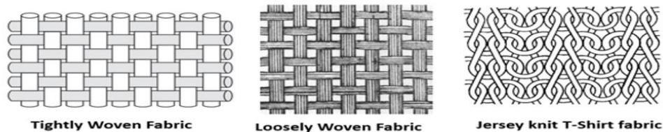
Figure 1. Typical drawings of tightly woven cotton fabric, loosely woven fabric and cotton knit jersey T-shirt fabric
