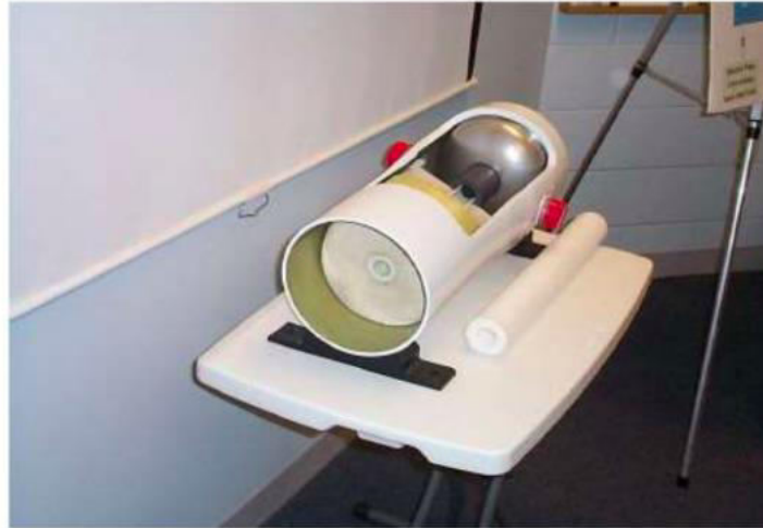
Figure 4. A cross-sectional view of a pressure vessel with a spiral-wound RO membrane
